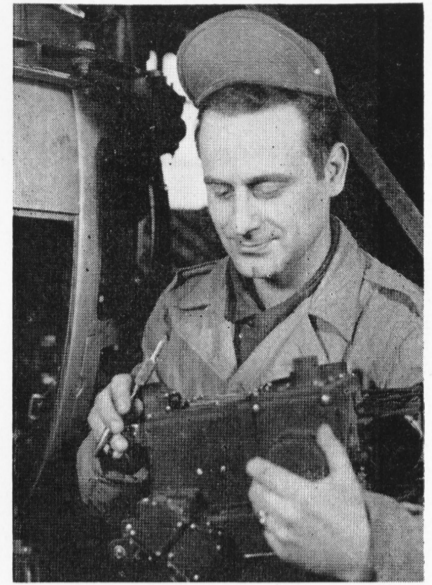
Staff Sergeant George E. Filley, formerly of Milling and Grinding, is now a turret maintenance engineer at an Eighth Air Force base in England. Here he makes an adjustment on a gun sight before installing it in the ball turret of a B-17 Flying Fortress.
